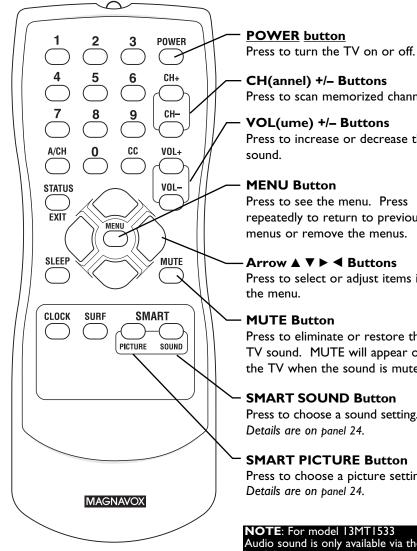
CH(annel) +/- Buttons Press to scan memorized channels. VOL(ume) +/- Buttons Press to increase or decrease the Press to see the menu. Press repeatedly to return to previous menus or remove the menus. **Arrow ▲ ▼ ► ◄ Buttons** Press to select or adjust items in Press to eliminate or restore the TV sound. MUTE will appear on the TV when the sound is muted.
